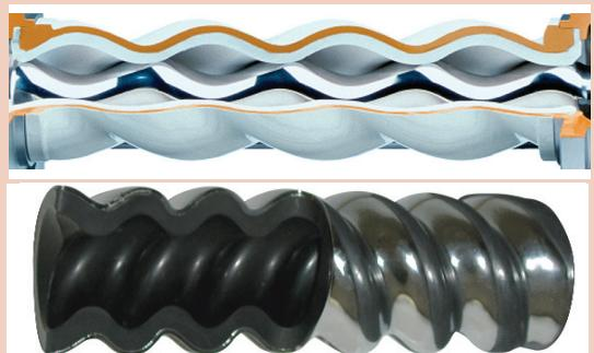
Even-wall stators can handle twice the pressure of conventional designs on non-abrasive fluids, with an even smaller footprint than conventional pc pumps. Both hysteresis failures and bond failures are practically eliminated.
